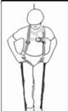
5. Stand onto the loop, so as to relieve the pressure of the harness webbing.
