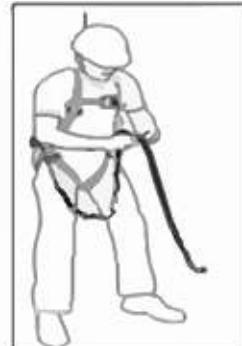
3. Connect the straps with each other making a loop with the help of the buckle.
