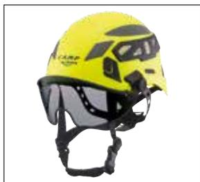
A ventilated helmet that satisfies the structural and functional requirements of both ANSI and EN standards. The robust ABS + polycarbonate shell features wide ventilation holes protected by metal mesh covers.
