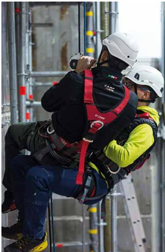
Two-person emergency descent test with a prototype of the Giant descender.
