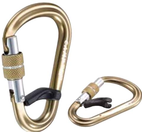
Aluminum alloy carabiner equipped with a proprietary internal lever that creates an inner ring that acts as a keeper for lanyards or energy absorbers. The system is designed to prevent unwanted rotation of the carabiner where it could be put in a compromised position.
